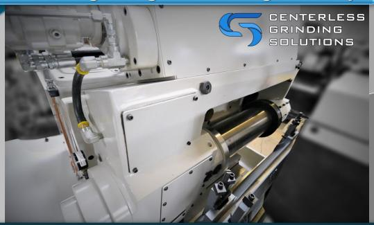
Complete Remanufactured Regulating Wheel Housing Assembly
