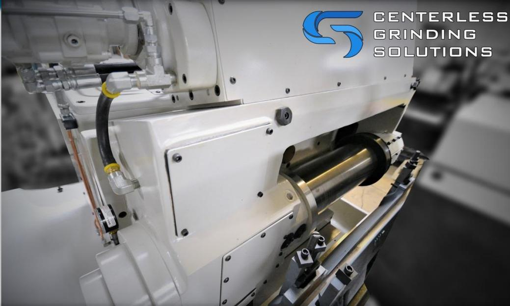
**Complete Remanufactured Regulating Wheel Housing Assembly**
